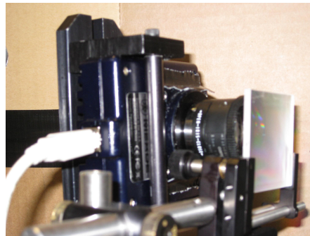
Fig. 5: Picture of Meade Deepsky Pro II imager and transmission diffraction grating setup
